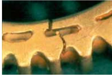
*Figure 11 Cracking due to silicon embrittlement in 18 carat gold [from reference (8)]*
