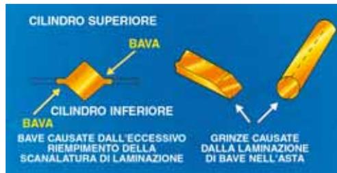
Figure 9 Schematic: Lap formation in rod rolling [from reference (10)]
