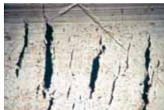
Figure 5 Cracking on the surface of ring made from continuously cast 14 carat gold [from reference (8)]
