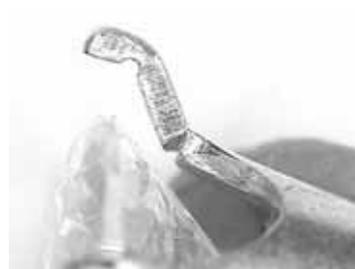
*Figure 12 Example of stress corrosion cracking in 14 carat gold [from reference (18)]*
