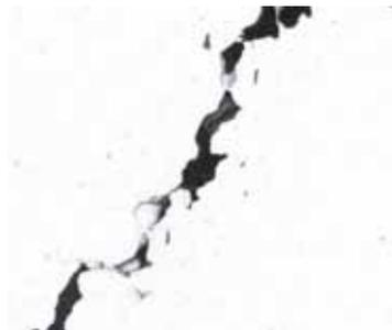
Figure 13 Quench cracking in investment cast silicon-containing 9 carat gold [from reference (19)]
