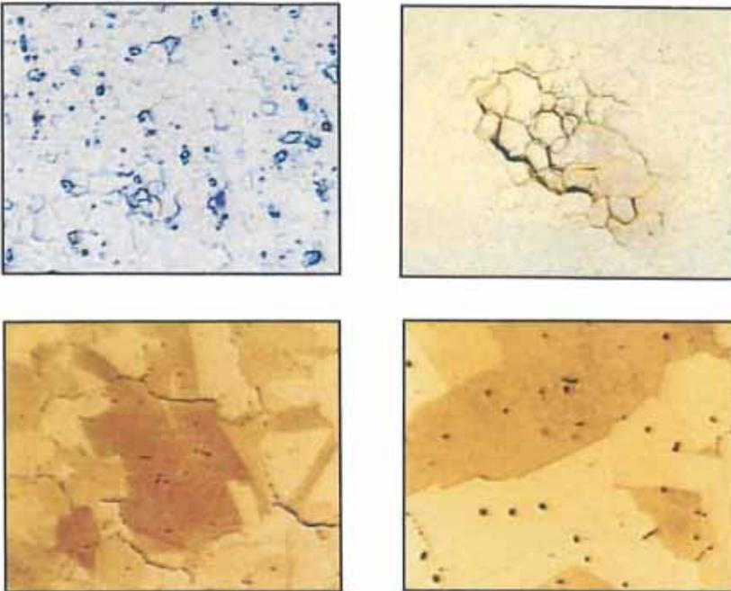
Figure 7 Porosity formation due to the 'steam' reaction in 18 carat gold: top – annealed surface; bottom – cross-sections 200x [from reference (8)]
