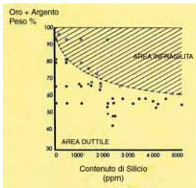
Figure 4 Effect of silicon content on embrittlement of carat golds [from reference (7)]
