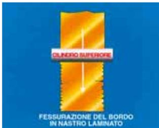
Figure 8 Schematic: Edge cracking in rolled strip [from reference (10)]
